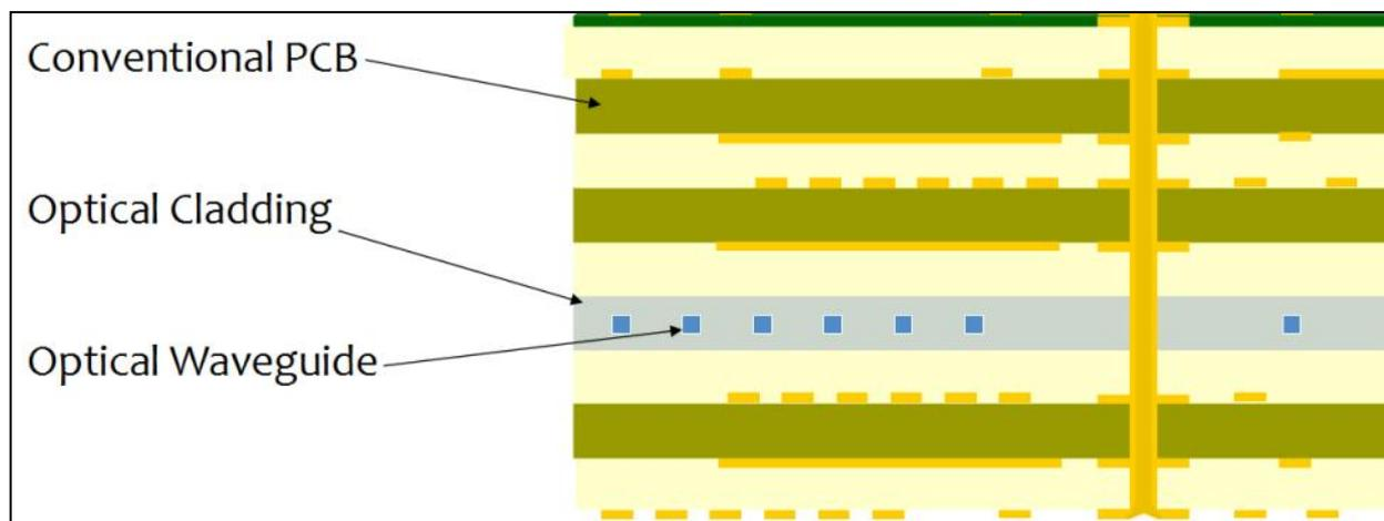
Figure 1 Proposed integration of optical waveguides in multilayer boards (source: TTM Technologies)
