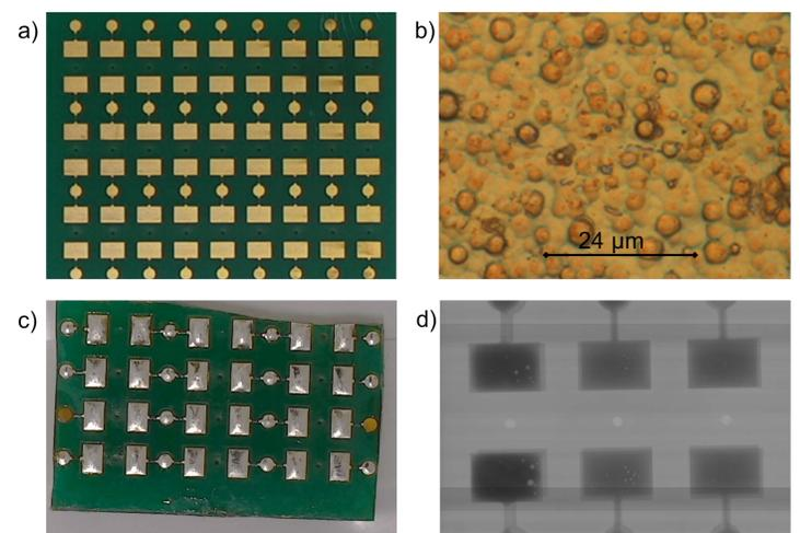
Figure 5: a) and b) Optical images of novel ENIPIG finish and c) and d) having undergone rotary solder wetting trials optical and x-ray image of soldered surface
