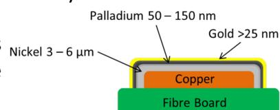
Figure 3: Cross section of ENEPIG coated PCB
